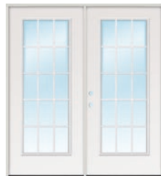
15-LITE DOUBLE STEEL #S21 U-FACTOR: .32 SHGC: .30 DT/VT: .31
