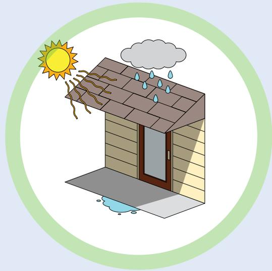
A proper overhang protects the door from direct exposure to sunlight, rain or snow – all day and from all angles. Lack of proper overhang will void the warranty and require routine maintenance.
