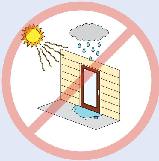
Direct sunlight and exposure to rain or snow will deteriorate the door finish. A proper overhang is required to protect the door from these elements. Lack of proper overhang will void the warranty and require routine maintenance.
