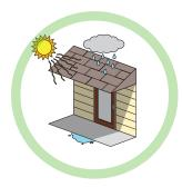
A proper overhang protects the door from **sunlight** on any part of the door, as well as rain or snow exposure. Lack of proper overhang will void the warranty and require **routine maintenance**.
