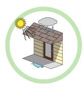
A proper overhang protects the door from **sunlight** on any part of the door, as well as rain or snow exposure. Lack of proper overhang will void the warranty and require **routine maintenance**.
