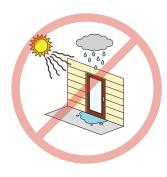
**Sunlight** on any part of the door, will deteriorate the door finish. A proper overhang is required to protect the door from sunlight, as well as rain or snow exposure. Lack of proper overhang will void the warranty and require **routine maintenance**.
