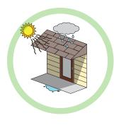
A proper overhang protects the door from **sunlight** on any part of the door, as well as rain or snow exposure. Lack of proper overhang will void the warranty and require **routine maintenance**.
