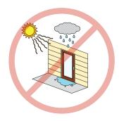
**Sunlight** on any part of the door, will deteriorate the door finish. A proper overhang is required to protect the door from sunlight, as well as rain or snow exposure. Lack of proper overhang will void the warranty and require **routine maintenance**.
