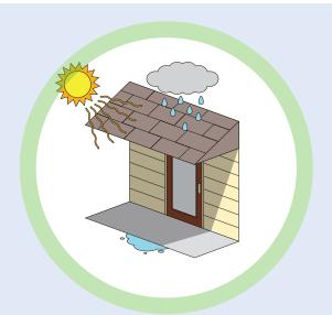
A proper overhang protects the door from direct exposure to sunlight, rain or snow – all day and from all angles. Lack of proper overhang will void the warranty and require routine maintenance.
