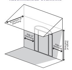
The "Projection of Overhang" must measure a minimum of 1/2 the height of the entryway. The "Side of Overhang" must measure a minimum of three feet from the outside edge of the door unit. The overhang must provide protection of the door unit from direct exposure to the elements.
